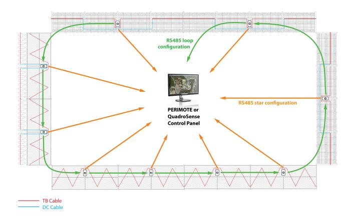
\*Instead of RS485 star configuration we can use common cooper wire to transmitt alarms from the receivers' dry contact f.e. to an alarm panel.
